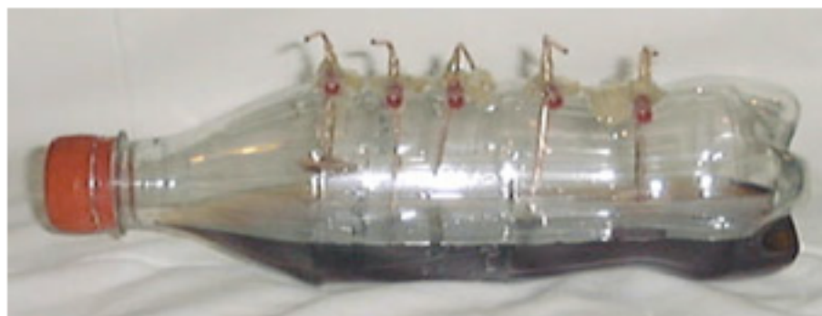
cola bottle plasma reactor with electrodes
