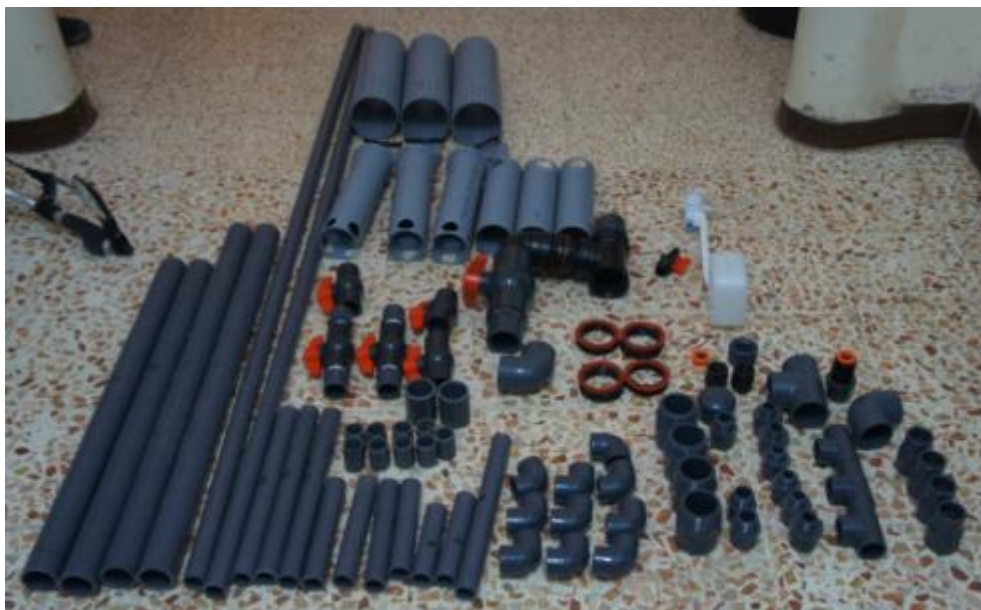
Figure 8: Plumbing components required for construction of the domestic scale aquaponic system
