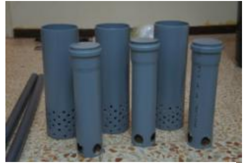
Figure 13: Siphon bell tubes (front) and shroud pipes (rear)
